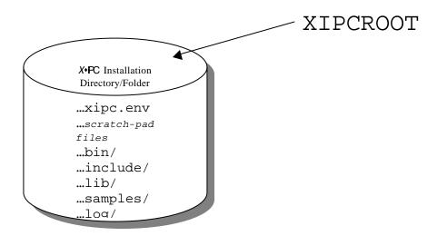
xipcinit's work includes the creation of a number of scratch-pad files within the XIPCROOT directory. As such, the XIPCROOT directory must be situated within a <u>writeable</u> area of the file-system.
