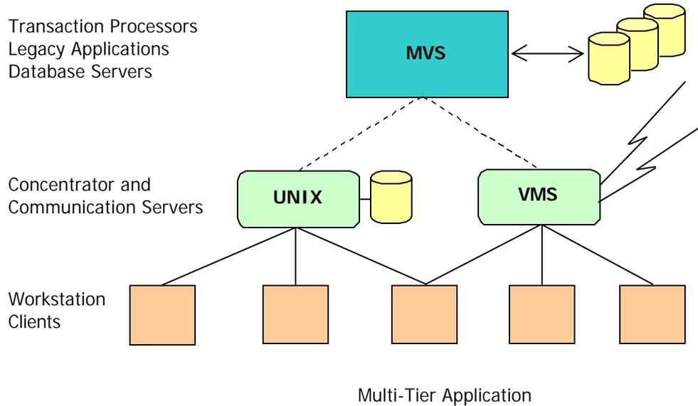
Such architecture is often associated with legacy applications that are being downsized into client/server distributed environments. Component processes in such architecture require the means for communicating, synchronizing and sharing data with each other in a generally asynchronous manner. Envoy XIPC's rich sets of asynchronous capabilities simplify the logical expression and coding implementation of such requirements.
